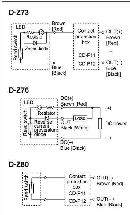
Note) A contact protection box should be used in any of the following conditions to prevent the shortening of the working life of the switch. (Refer to page 40 regarding the detailed specification for contact protection box):
