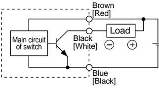
(Power supplies for switch and load are separate.)
