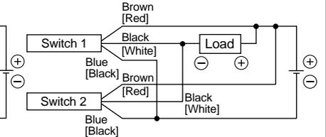
The indicator lights will light up when both switches are turned ON.
