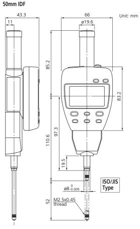
Note: Dimensions of the ANSI/AGD (inch/metric) type IDF indicator partly differ from those of the ISO/JIS (metric) type IDF.
