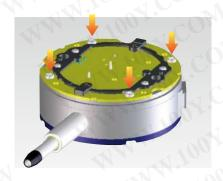
Greater rigidity in the bearing plate for reduced retrace error (20%) and 4-screw mounting for increased impact resistance.
