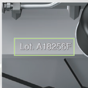
Presence inspection of marked characters
