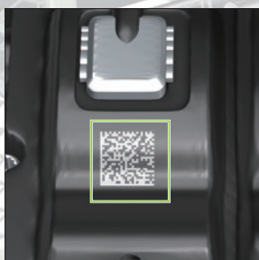
Reading direct part marks
