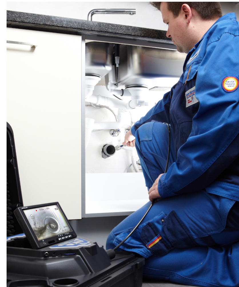
Waterproof up to 3 bar, robust colour camera head with Ø 26 mm can be pushed through several 87° bends into pipes of Ø 40 mm.
