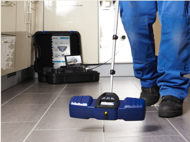
Digital indication of the electronic metre counter on the display. Radio localisation possible with the Wöhler L 200 Locator.
