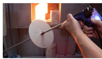
**Easy to attach:** Our heat protection shield ensures your safety and the safety of your device while measuring at high temperature spots of up to 1,200 °C. Additionally, you have the flexibility to measure at various spots by extending the probe from 1 m to 2 m if needed
