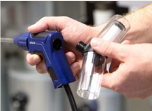
CHP filter: The CHP filter protects the sensors when measuring CHP or solid fuel systems.
