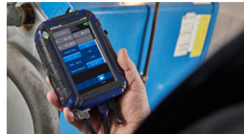
5" large colour touchscreen: All measurement and calculation values at a glance - Simple operation via touch display - Structured menu navigation.
