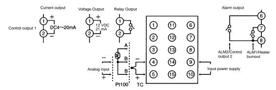
Two input power supplies are available: 100 to 240 VAC or 24 VDC.
