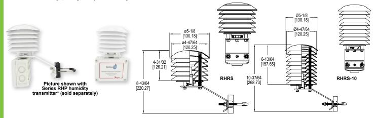
The Series RHRS Outside Air Humidity Radiation Shields protects outside air humidity transmitters from rain and radiated heat. With the curved shape and color of the plates, air flow is able to move across the sensor to keep radiated temperatures from rooftops and surrounding surfaces from affecting humidity readings.
