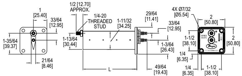
The **Series MAFS Metal Averaging Flow Sensor** is ideal for use with Dwyer® precision air velocity gages, transmitters and switches. The Series MAFS uses evenly distributed total and static pressure measuring points to deliver an accurate measurement of velocity pressure in a duct.
