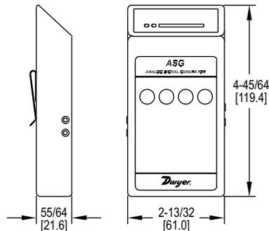
The **Model ASG Analog Signal Generator** generates a 0-10 VDC signal in increments of 1 V or a 4-20 mA signal in increments of 2 mA. An LED bar graph visually indicates the analog signal level. Model ASG will also continuously ramp to user defined maximum and minimum values with user defined ramp interval timing.
